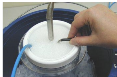
Ice bath calibration of temperature sensors
